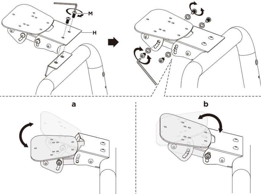
**7** Racing Seat: Height & Tilt Adjustment
